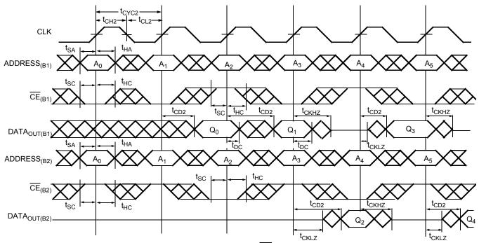
Figure 10. Read-to-Write-to-Read ( $\overline{OE}$  = LOW)<sup>[36, 39, 40, 41, 42]</sup>
